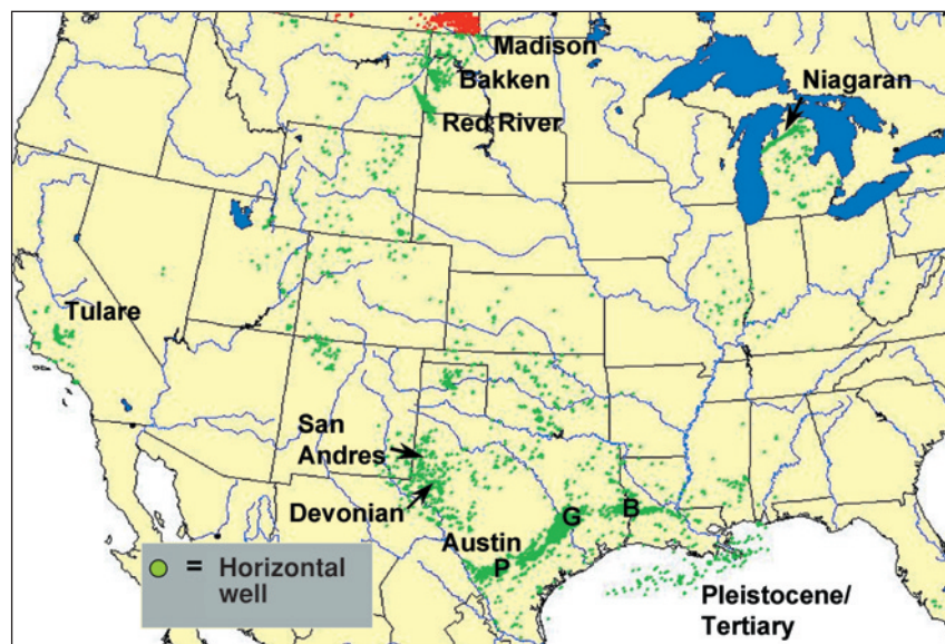
FIGURE 3. Map showing horizontal wells in the United States and southern Canada. Data extracted from IHS Energy Group databases as of May 1999. Leading reservoirs and fields for horizontal wells are annotated. P = Pearsall field; G = Giddings field; B = Brookeland field.
