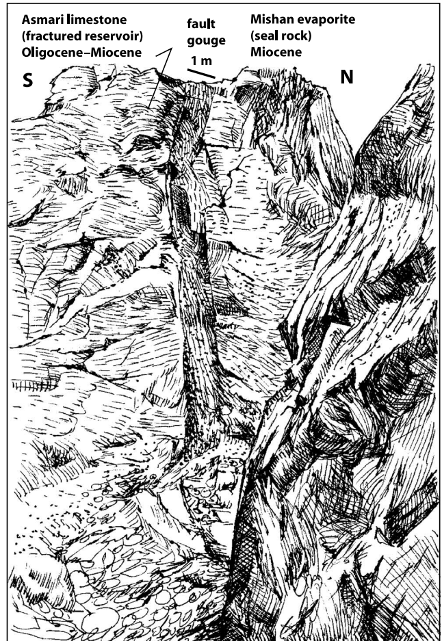
FIGURE 6. The Khurgu fault in the Zagros foreland basin, southern Iran. Fault juxtaposition of Asmari limestone (a major reservoir rock in the subsurface) against Mishan anhydrite (a regional seal rock) with intervening fault gouge (about 1 m [3 ft] thick). In such juxtaposition traps, the higher capillary pressure of either juxtaposed seal rock or fault rock determines the sealing capacity of the fault. This high-angle reverse fault was not reactivated in the 1977 Khurgu earthquake (magnitude 7). Drawn from a photograph in Berberian et al. (1977).
